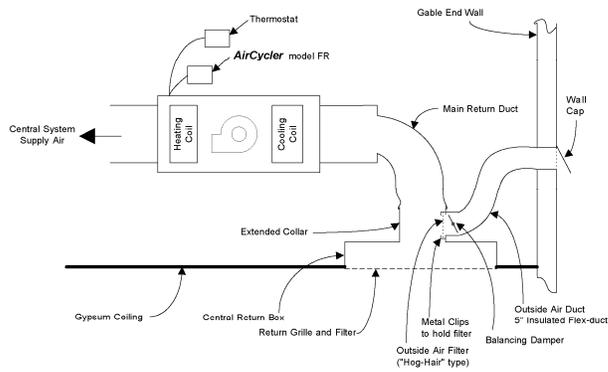
**Figure 1: Central fan integrated supply system (shown with horizontal attic mounted unit as example)**
