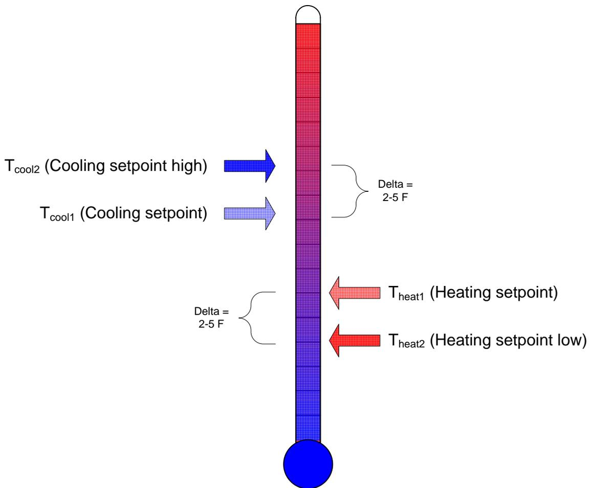
**Figure 3: Schematic relationship of heating and cooling setpoints**
